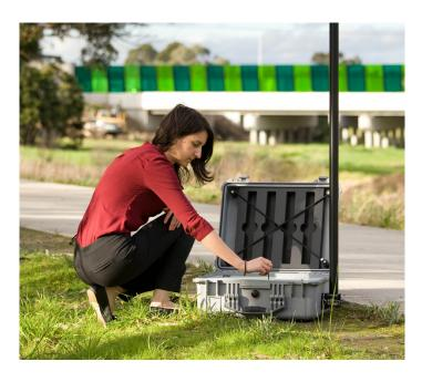
The logger includes Hand-held Analyzer Type 2250 and all of the software and accessories you need to complete your monitoring project, including full statistics, 1/3-octave band analysis, audio recording with event triggering and a memory card.
