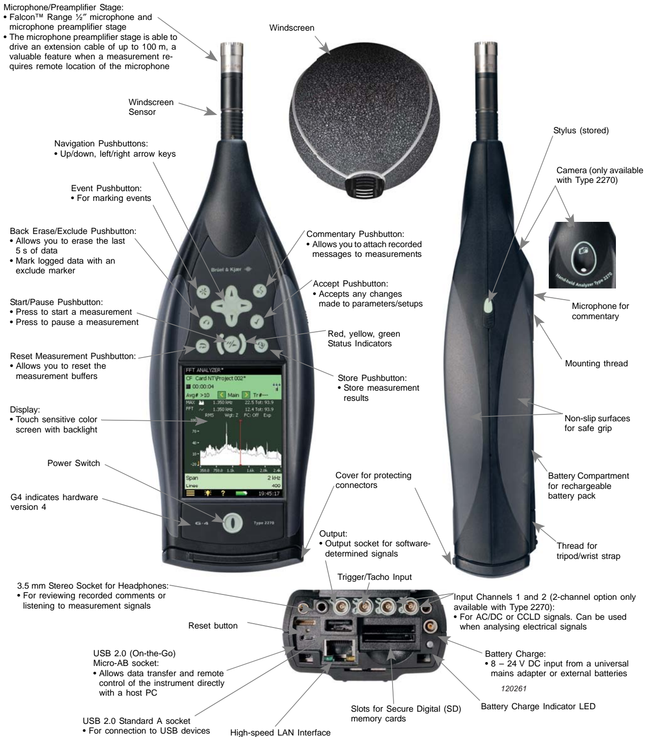
Fig. 1 Key features of Hand-held Analyzer Types 2250 and 2270
