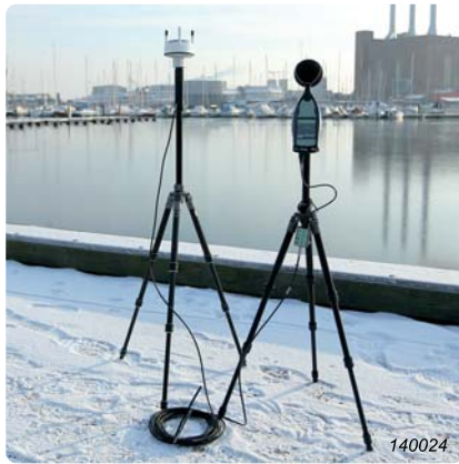
Fig. 12 Hand-held analyzer measuring outdoor noise using Weather Station Kit MM-0316-A
